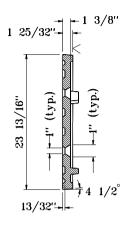
1" dia. anchor bolt holes on a 29 1/8" dia. b.c. 4 reqd.
